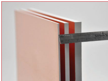
▲ Fig. 1 Laminates can have different dielectric constants, panel thicknesses and copper claddings.
